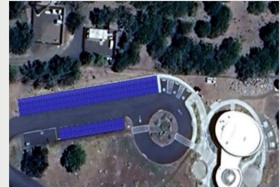
Goldendale Observatory Carport Array: 125.0 kW Cost per Watt = $18.50
