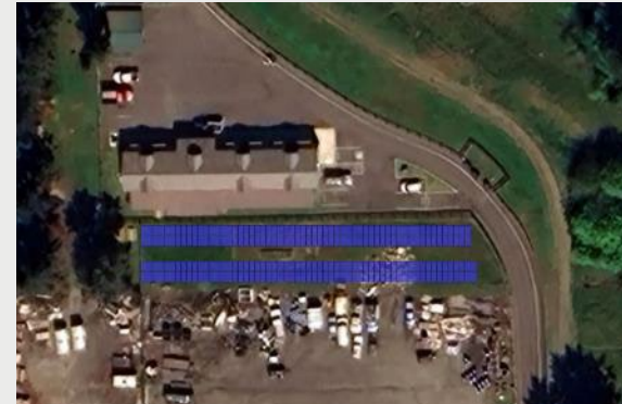
Fort Worden Shop Complex Ground Array: 127.0 kW Cost per Watt = $13.60
