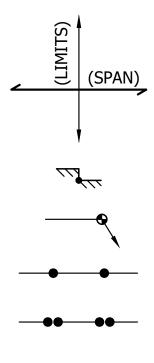
GRATING OR STRUCTURAL SPAN DIFFERENCE IN ELEVATIONS ELEVATION TARGET (REF.) HANDRAILING REMOVABLE HANDRAIL
