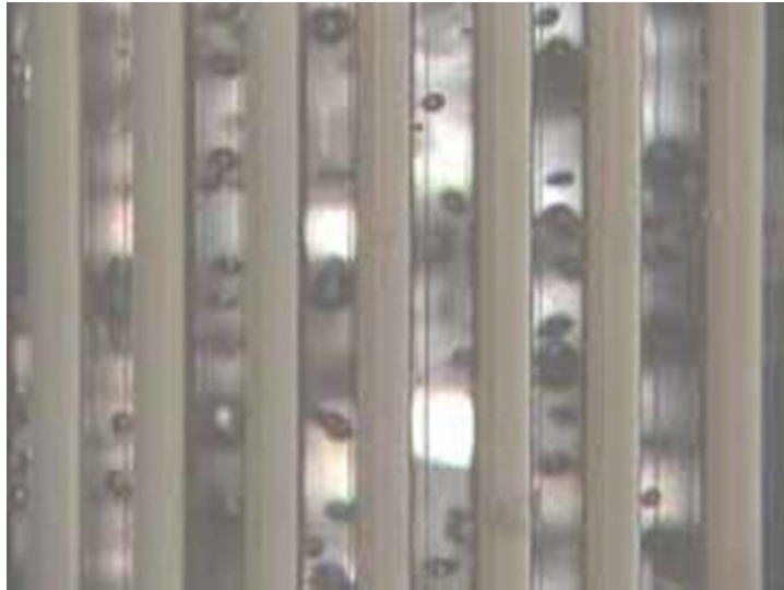
Figure 2: Fixed spacing between each membrane cartridge provides efficient air scour
