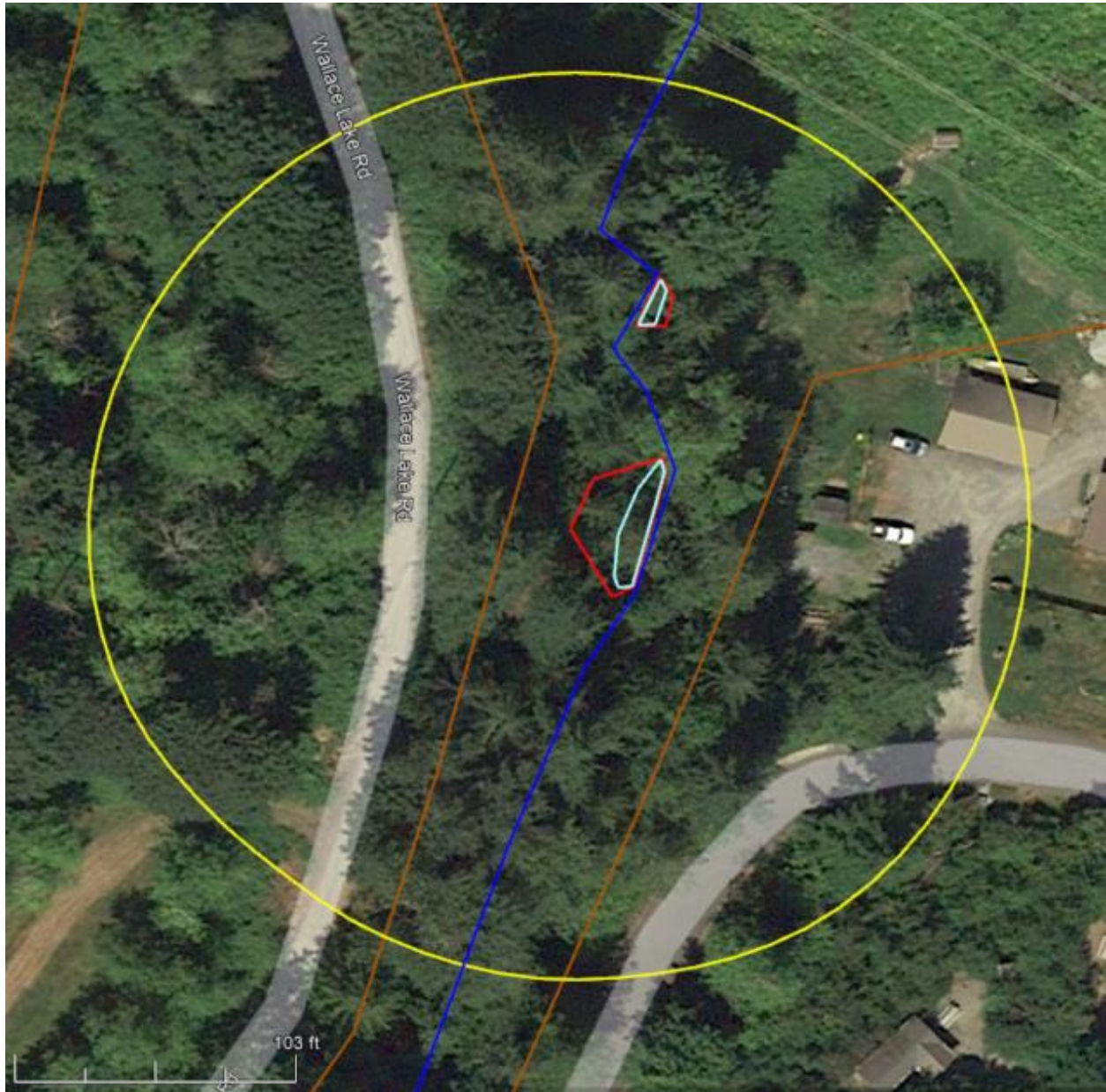
Figure 1. Detail of Cowardin Classes for Wetland W1 above and W2 below. Red outline is the wetland and yellow is 150-foot boundary. Hydroperiods are seasonal flooding indicated by blue (remaining area is saturated), and permanently flowing stream. Wetland Cover is PSS with upland over canopy of trees. The outlet for wetlands is the interface of the wetland with the stream.
