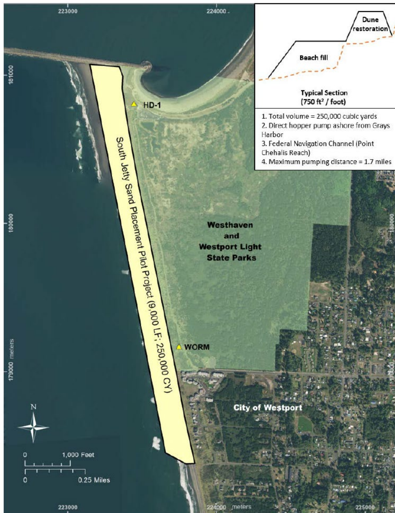
Figure 5: Proposed Grays Harbor South Jetty Sand Placement Pilot Project Area, with the location of two long-term beach profile locations shown for reference
